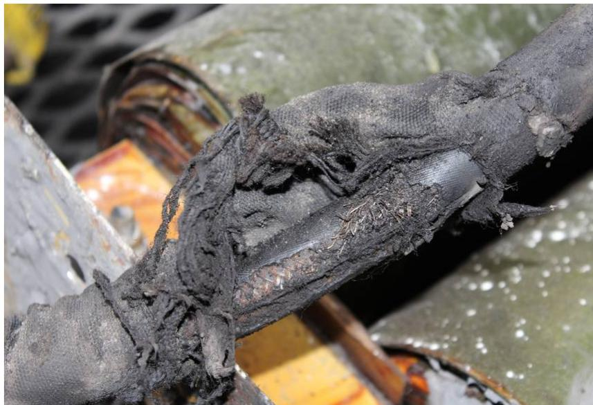
*Figure one – Hose failure through external wear and abrasion*
