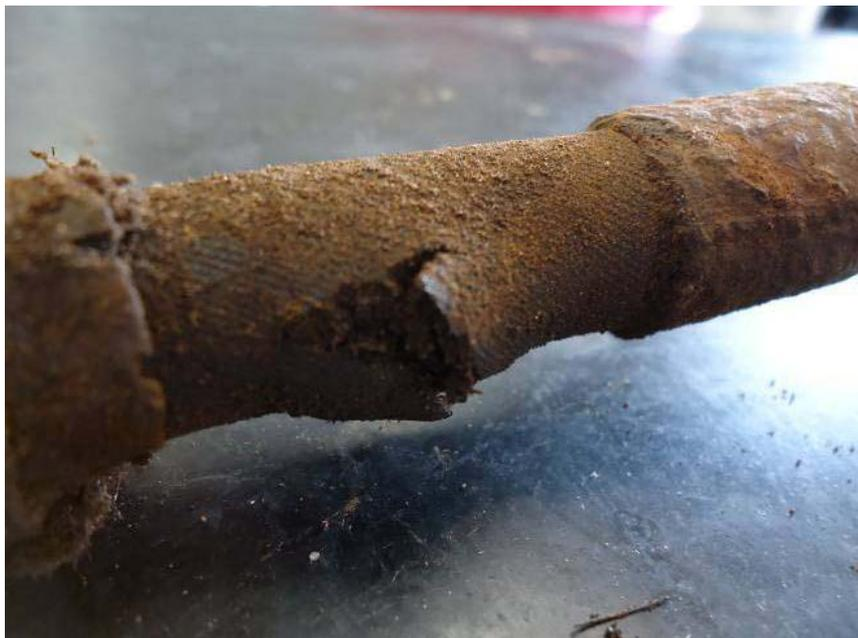
*Figure two – Hose failure through corrosion and too tight bend radius*
