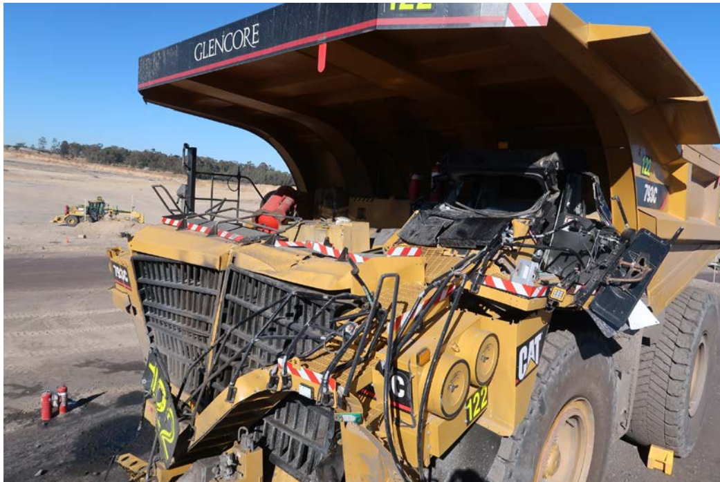
Figure 2: Damage to front and cabin of DT122
