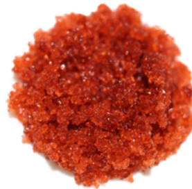
Battery ready cobalt sulphate from Thackaringa. Image courtesy of Cobalt Blue Holdings Limited.
