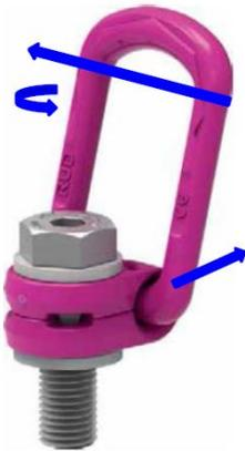
Figure 5: Direction of loading to cause deformation observed
