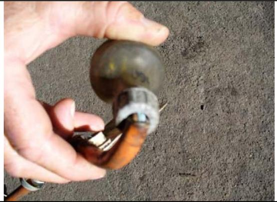
Defective cable connection to the plug
