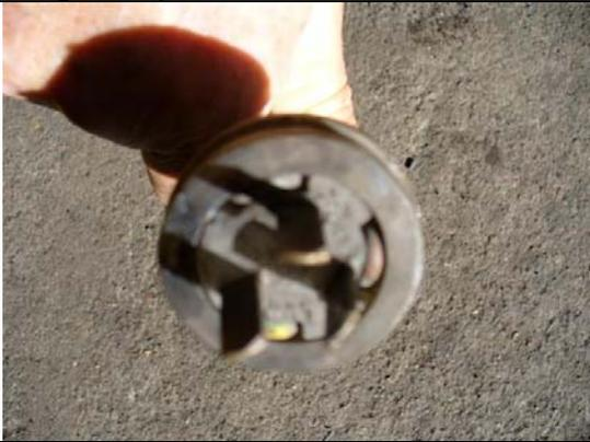
Plug inadequately IP-rated
