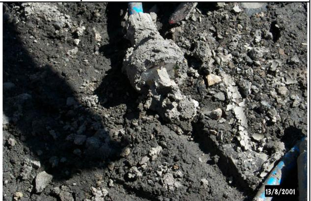
Plug not suitable for the environment, poorly installed and poorly maintained
