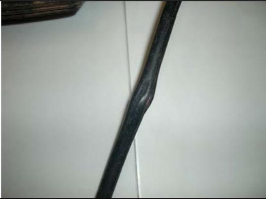
Damaged impact wrench lead
