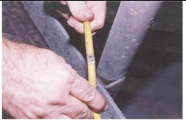
Damaged extension lead due to poor installation practices.
