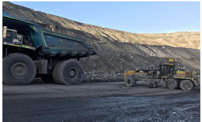
*Figure 2 Contact between haul truck and grader*
