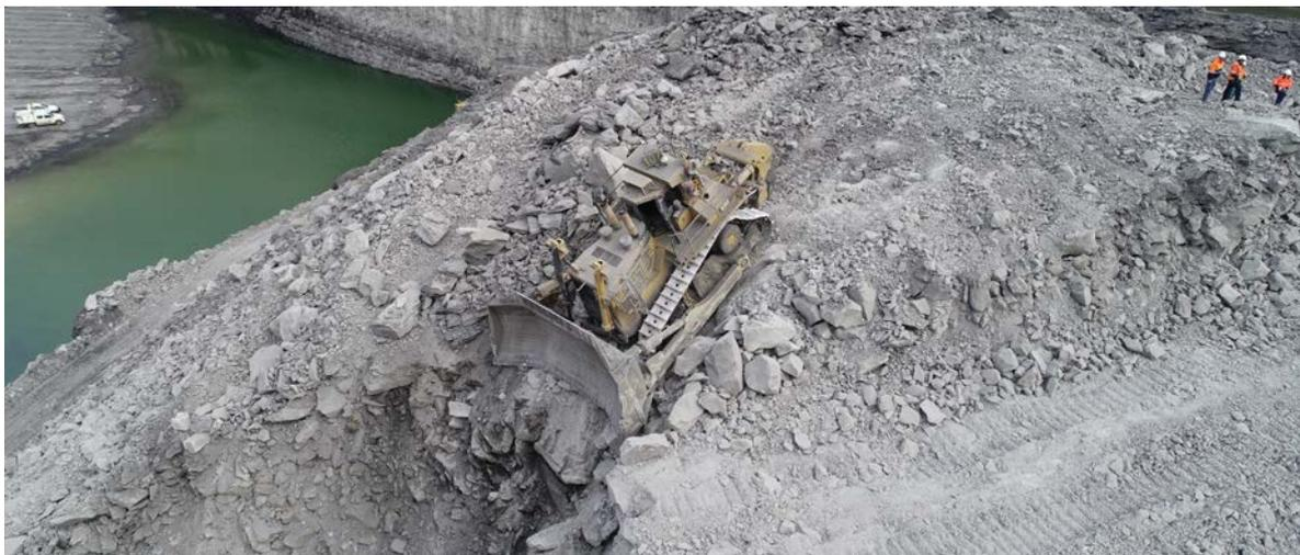
Figure 2 Dozer rolled while reversing at a metalliferous mine
