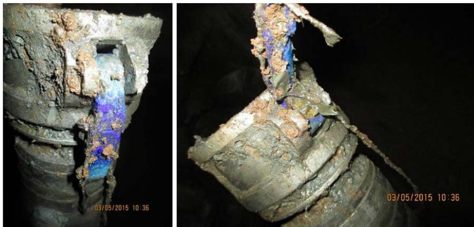
Image 1 - TACN on brass locking lever of cam-lock
