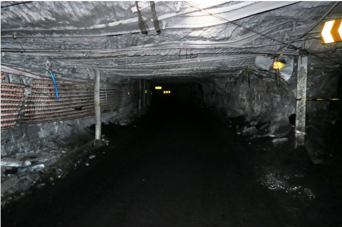
Photograph of roof support straps (W Straps) in the travel roadway. *Photograph taken by investigators.*
