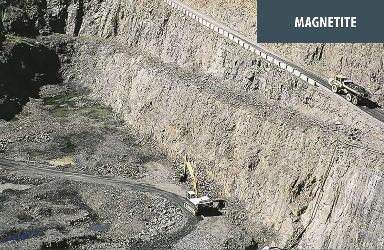
*Photograph 15. Tallawang magnetite mine, Gulgong. The Tallawang mine is the sole producer of magnetite in the state. The magnetite is used almost entirely by the New South Wales coal mining industry during coal beneficiation. When finely milled, magnetite remains suspended in water, producing a dense medium suitable for separating impurities from coal. The magnetite is easily recovered by applying a magnetic field. (Photographer I. Paterson)*
